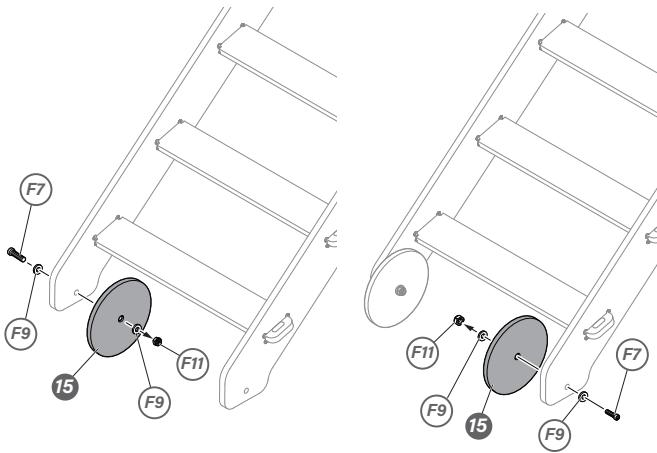
**21** Secure the ladder using clevis pins
